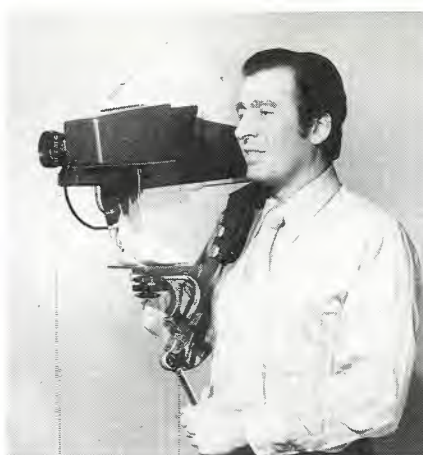
RCA's unique entry has a miniature viewfinder. Note the far-forward mainstructure positioning.
