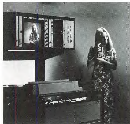
Unveiled at the show was the Ampex modular AVR-2 VTR. It can be quickly dismantled and carried out to a remote site. It weighs about 600 lbs.
